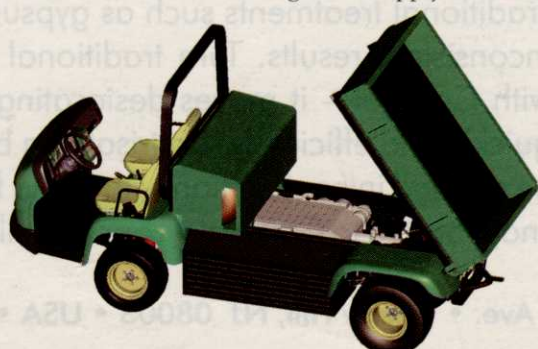
An engineering diagram of Deere's hydrogen-powered Pro-Gator
