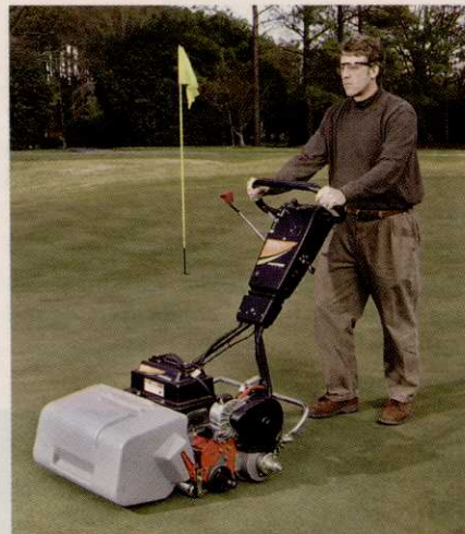
The E-walk has two 48V electric motors
