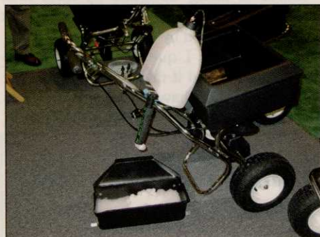
The foam marking kit on a Spyker spreader
