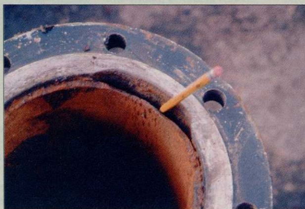
An acid-eaten section of pump station piping
