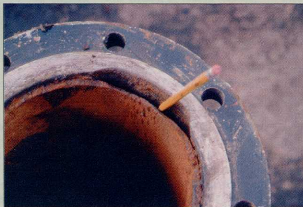
An acid-eaten section of pump station piping
