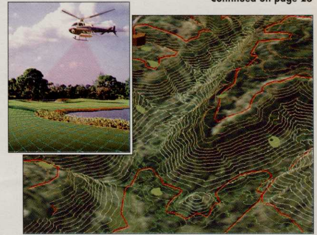
LiDAR mapping generates detailed topographic maps using lasers (above) attached to a helicopter deployment platform (inset).
