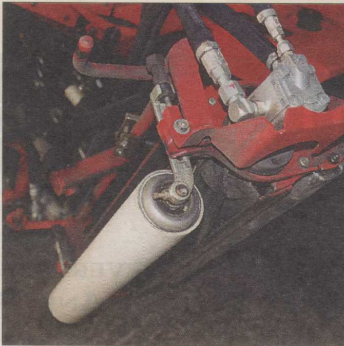
PVC piping can turn a Whiele roller into a solid roller in a matter of minutes.
