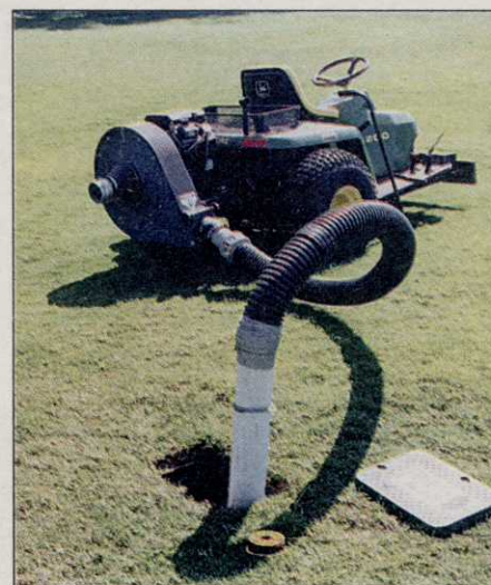
Olde Florida Golf Club demonstrates the effective use of existing equipment with a separate engine-powered blower. The blower can be used elsewhere, such as to blow debris from inside a bunker.
