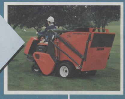
Most efficient pick-up of even the smallest debris Sweeping reel with flexible fingers rides on castor wheels that closely follow terrain and prevent any damage to turf Polyester screen filtration system removes over 90% of the dust and dirt for maximum safety and comfort for the operator
