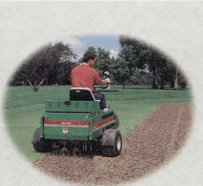
GA™ 30 —A combination of variable core spacing, speed and precision coring. Aerate greens, tees and fairways up to a depth of 3.75 inches.
