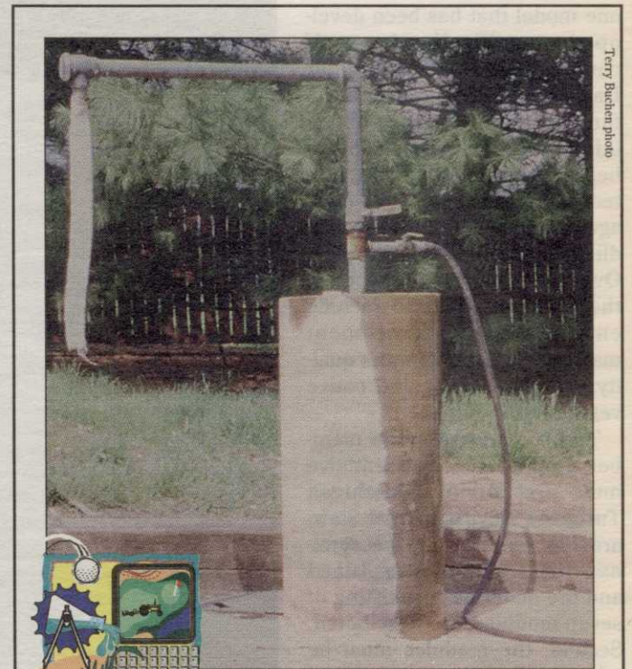
Filling a truckster-mounted or towable sprayer with water is easier with this simple devise.
