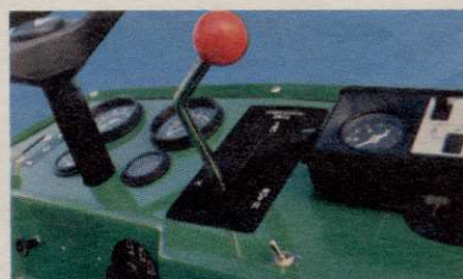
A single lever hydrostatically controls the 1800's direction and speed.
