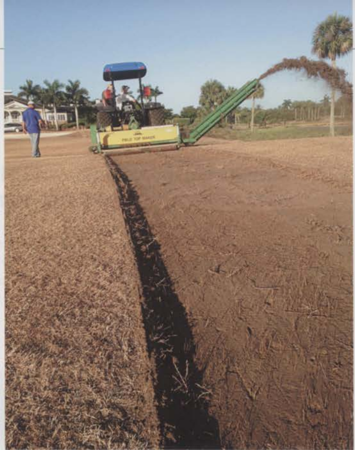
The Koro rototiller in action on The Rookery's fairways during renovation. Note how deep the tiller goes to remove the old turf layer. Photo by Todd Evans.
