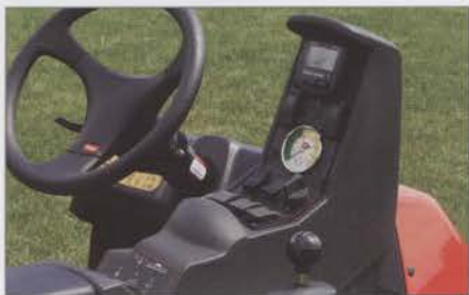
The QuickFind Console intuitively helps the operator find boom and actuator switches without looking at them
