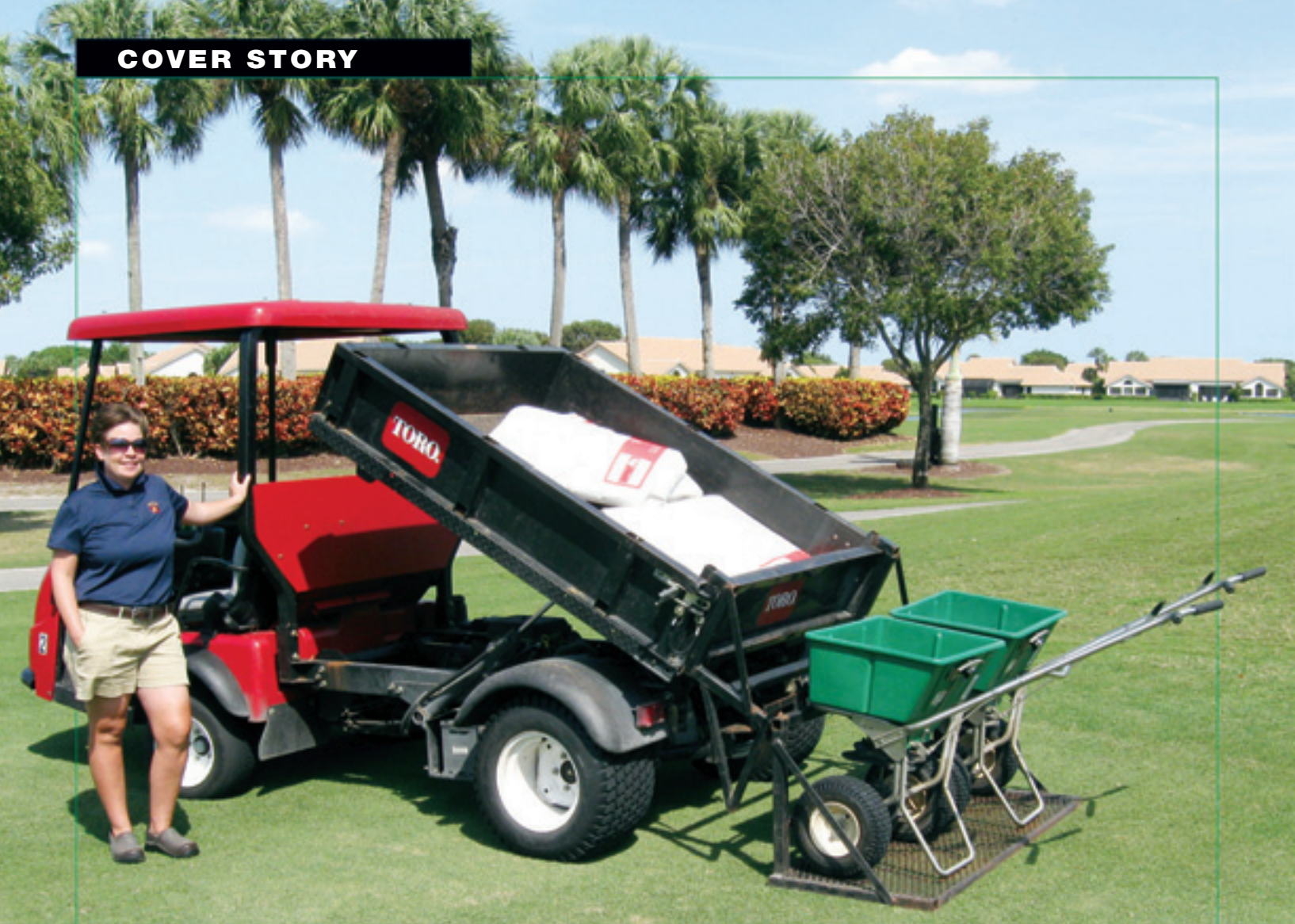
First Assistant Angela Wilson shows off a back saving spreader rack idea that Brian brought home from a trade show. Photo by Joel Jackson.
