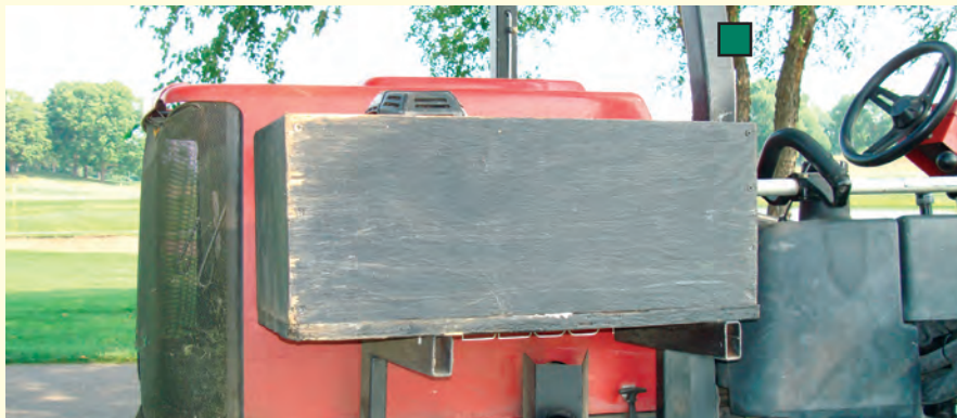
Close up of the plywood box and bracket attachment housing the motor part of the string trimmer. Photo by Darren Davis.
