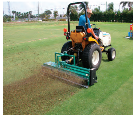
Art Lewis of Lewis Equipment demonstrates a verticutting unit during the South Florida Turf Expo. Photo by Joel Jackson.
