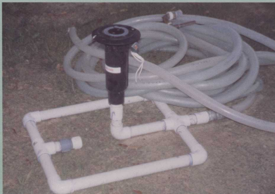
Easy and affordable to construct, this portable 1-1/2-inch PVC base is stable and delivers extra irrigation where needed at optimum pressure. Photo by Darren Davis.
