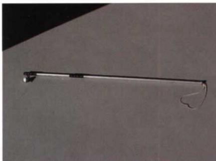
An effective snake-handling tool can be made from an old dew whipping pole, some starter cord and a golf ball. Photo by Bill Davidson, Jr.
