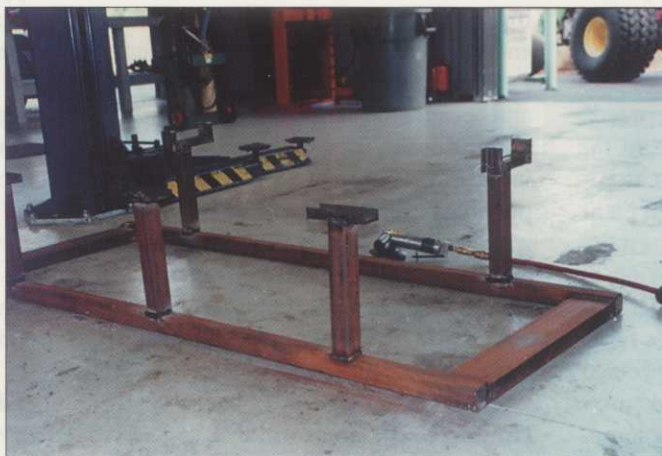
Note the three rear risers with the parallel C channel cradles and the two front risers with the perpendicular cradles. Photo by Darren Davis.
