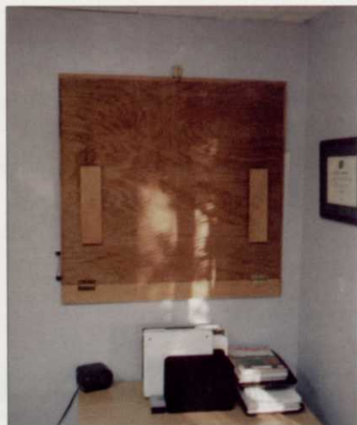
The blueprint board folded up flat against wall in storage position.
