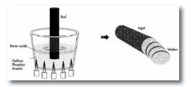
solution and pulled out slowly. The solution cools and crystallizes on the end of the rod as it is lifted out of the chamber, forming a long, cylindrical crystal ingot. The ingot is then sliced into wafers. Each of the semiconductor materials (called substrates) and impurities result in various colors of light from the LED.
