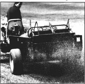
In one easy step, eliminate costly dumping fees and improve the rough by spreading grass clippings still enriched with precious fertilizer. Millcreek's Top Dressers are equipped with an adjustable undershot poly brush designed to evenly distribute top dressing from three to ten feet wide.
