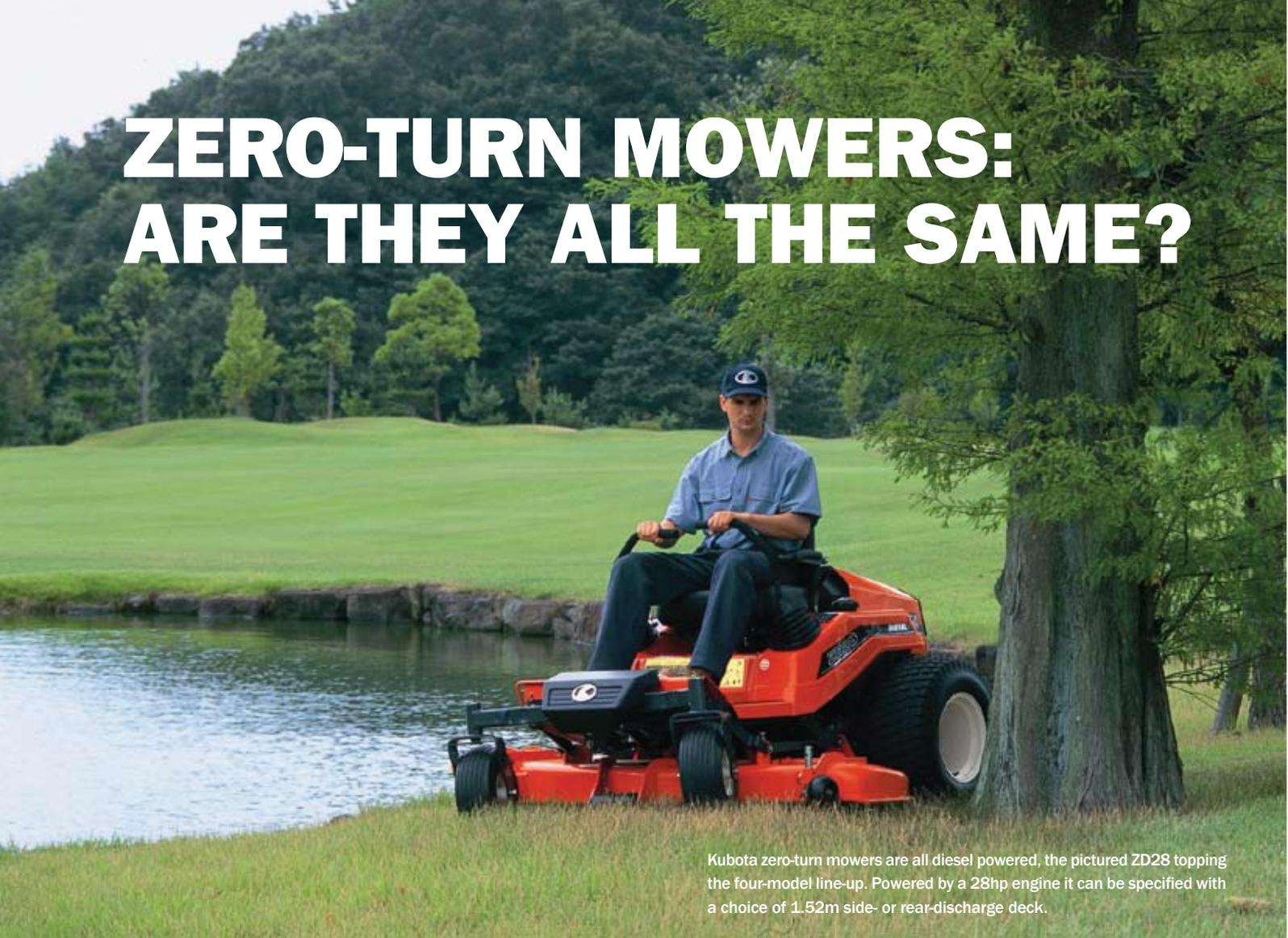
Kubota zero-turn mowers are all diesel powered, the pictured ZD28 topping the four-model line-up. Powered by a 28hp engine it can be specified with a choice of 1.52m side- or rear-discharge deck.
