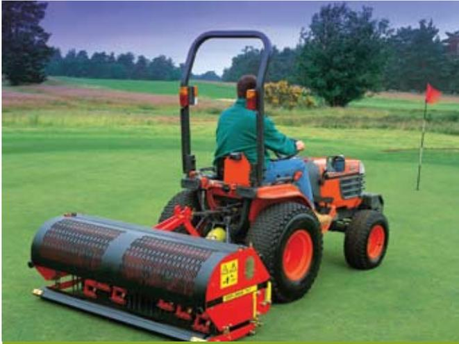
Forward speed can be absolutely critical for some jobs, so it is important to choose a tractor with the ability to deliver the right pace at rated PTO speeds. Equipment manufacturers can often suggest a good tractor for the job.
