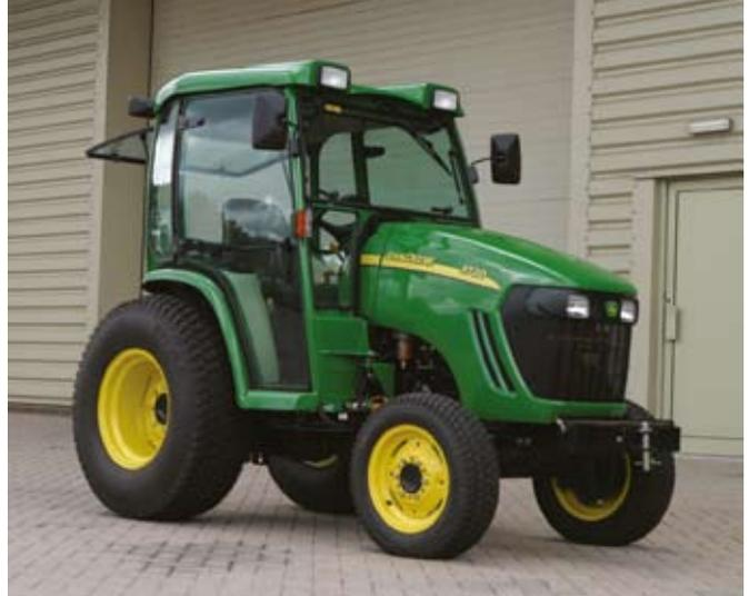
Developing 44hp, the John Deere 3720 has an easy to use hydrostatic transmission. A tractor of this type can be used with fixed speed kit, but a manual shift is often the preferred choice for this type of work.
