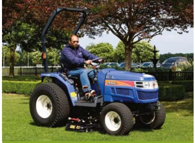
Developing 29hp, the Iseki TH4290 is another hydrostatic drive model that can readily be specified with a mid-mount deck. Hydrostatic transmissions are ideal for mowing work.
