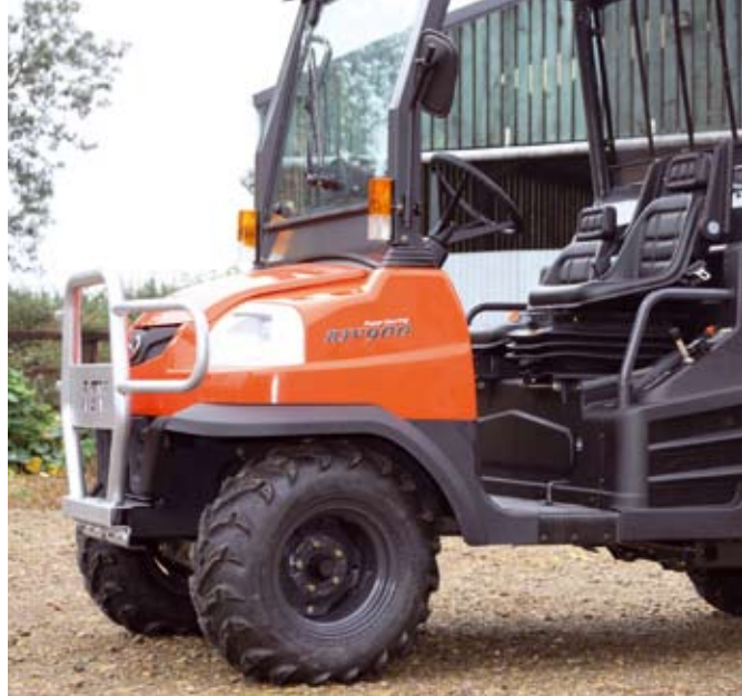
Road homologation is another feature offered by manufacturers to include Kubota. With its hydrostatic transmission and power steering, the RTV 900 is currently unique.
