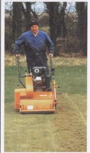
It incorporates the SISIS Rotorake contra-rotation principle, whereby the reel rotates at high speed against the direction of travel. The blades therefore cut upwards continuously throwing fibre forwards rather than pushing it into the surface. The machine is also held to the ground to maintain a regular working depth.
