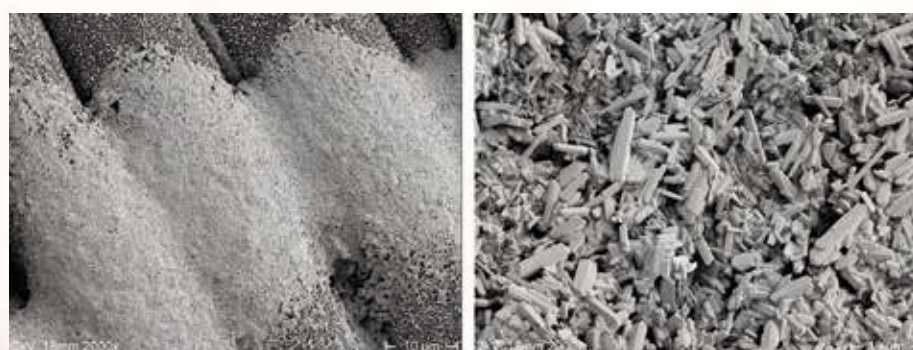
Plate 1. The finely milled formulation of Medallion TL (left) is better able to bind onto the wax layer of the leaf surface to provide seamless coverage, compared to blocky particles of an iprodione fungicide, for example.
