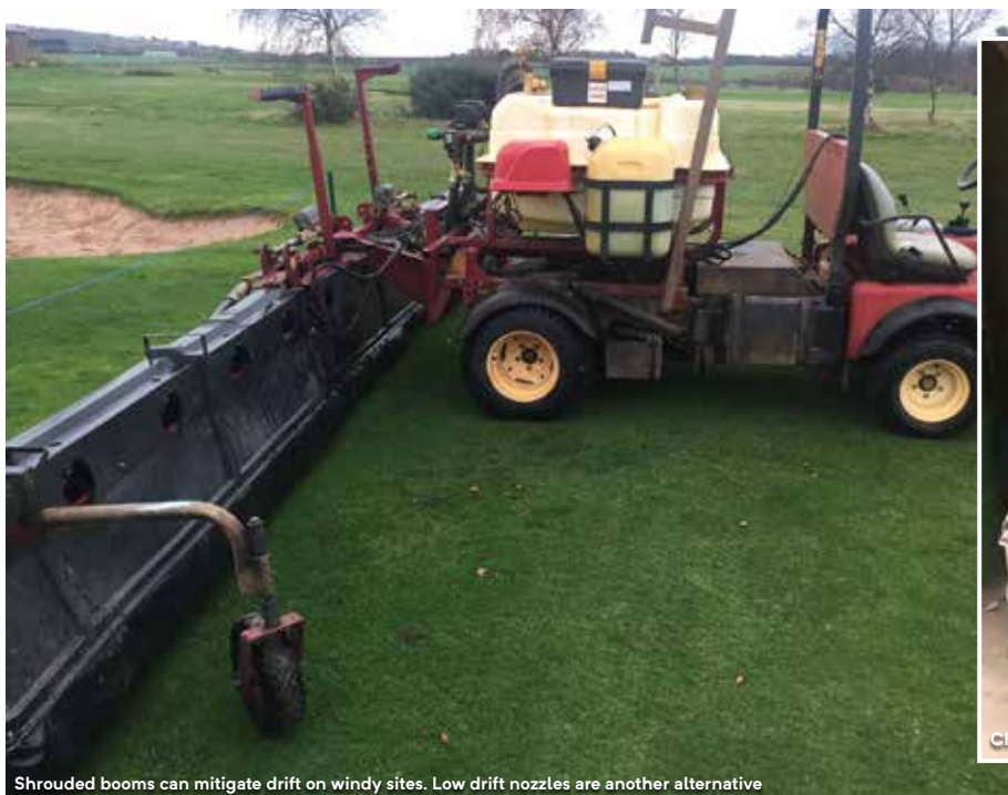
Shrouded booms can mitigate drift on windy sites. Low drift nozzles are another alternative
