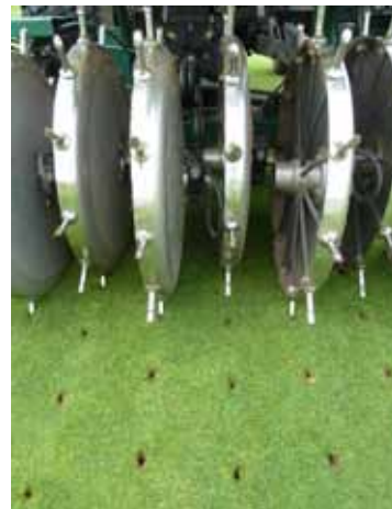
ABOVE: Close-up on turf injection with the Liquiject 760 at Hart Common.
