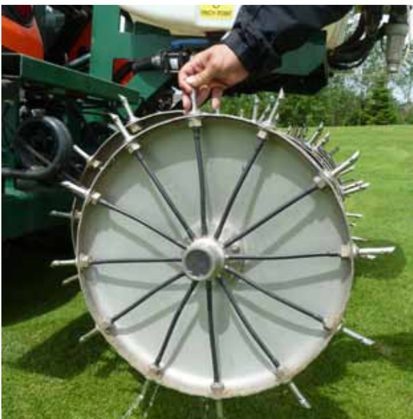
The Liquiject system injects liquid formulations precisely and accurately down into the root zone with a minimum of turf disturbance.
