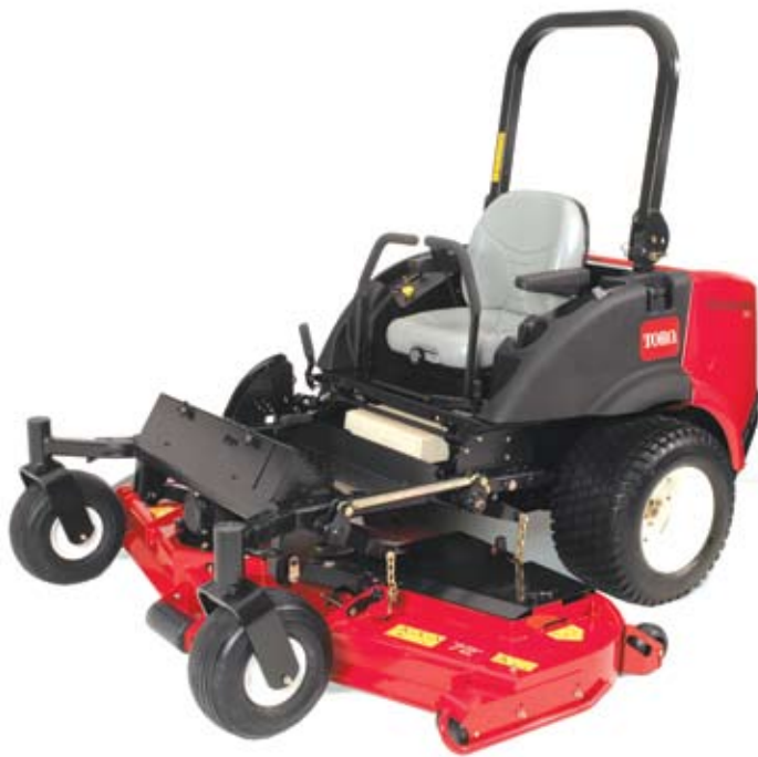
Toro Groundsmaster 7200 series 28hp zero-turn mowers can be fitted with a choice of decks, including 1.58 and 1.83 Guardian recycler units. Made from heavy steel, the decks are claimed to be extremely tough and leave a really good finish.
