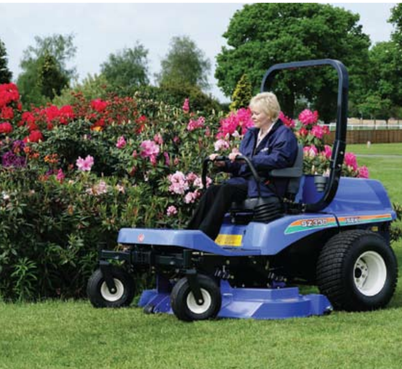
The 33 hp Iseki SZ330 is among the most power zero-turn models, its large 1.83m deck enabling it to match tight turning with a high level of productivity. Large driving and big front castor wheels useful for work on rougher ground.
