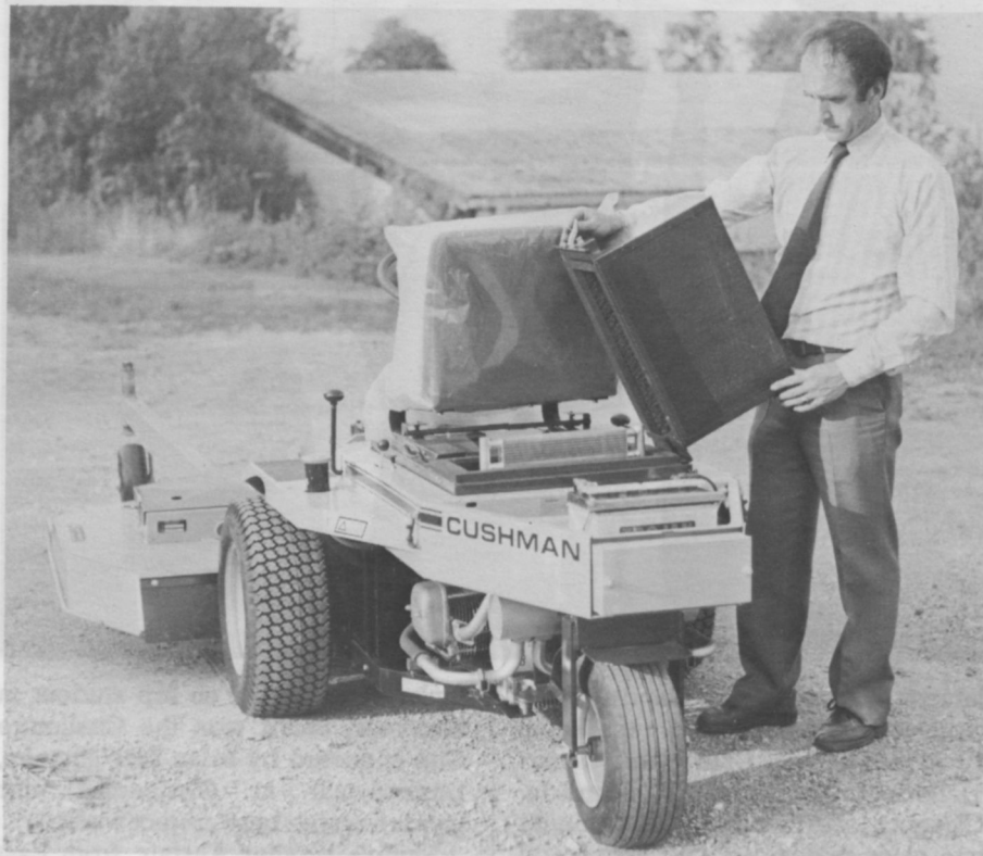
Cool, clean air is ducted to the Cushman Front Line's petrol engine via a compact filter screen mounded behind the driver's seat. The new air intake filter, which also houses the transmission oil cooler, can be easily removed for cleaning.
