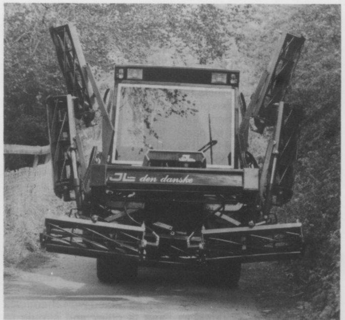
The new JL Multi-Trac equipped with a seven gang, hydraulically-driven gang unit.
