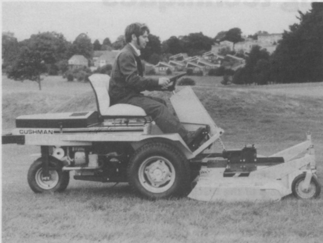
The New Cushman Front Line now has a full range of interchangeable front implements for mowing, sweeping and snow clearing.
