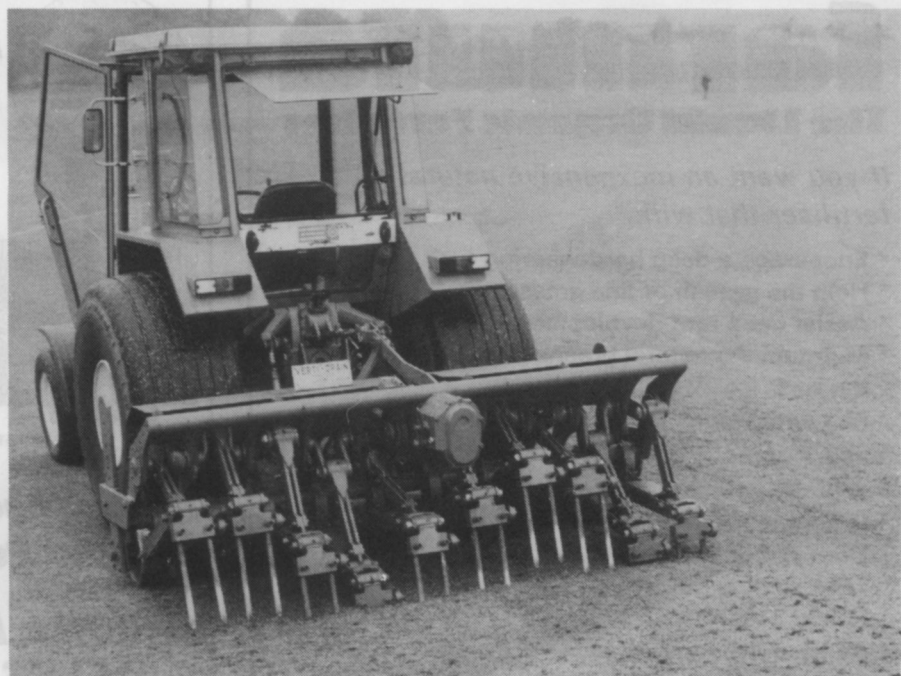
The Verti-Drain in operation.
