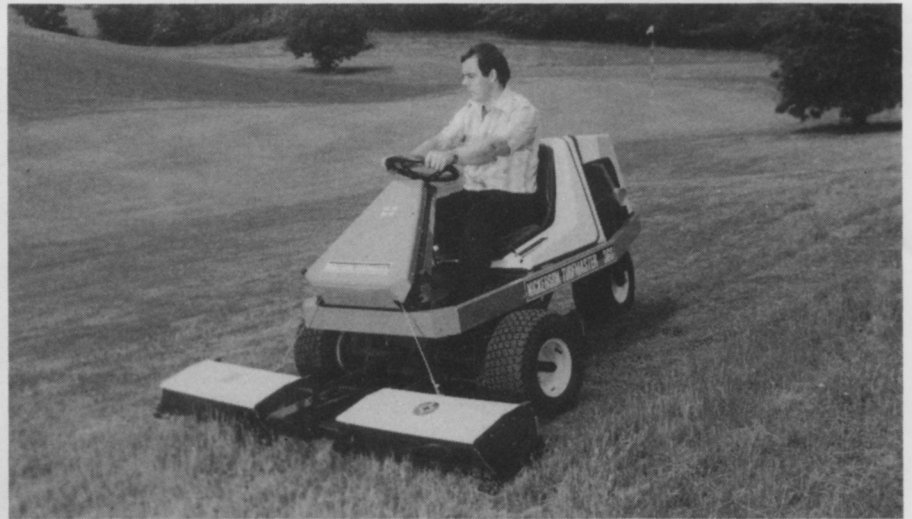
The new Nickerson Turfmaster 360, which features three cylinders and has a maximum cutting width of 70 inches, is ideal for the cutting of tees, approaches and backs of bunkers.
