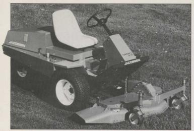
Another convenience of the HF-15 is that its reels are hydraulically powered making the cutting frequency pre-set by the operator independent of the unit's speed. The operator's seat is fully padded and adjustable and controls are situated to keep a person safety in a seated position. Levers for raising and lowering cutter decks and reels are within easy reach. Cabs available for the Turfcats and the HF-15 have positive ventilation systems to keep dust out.
