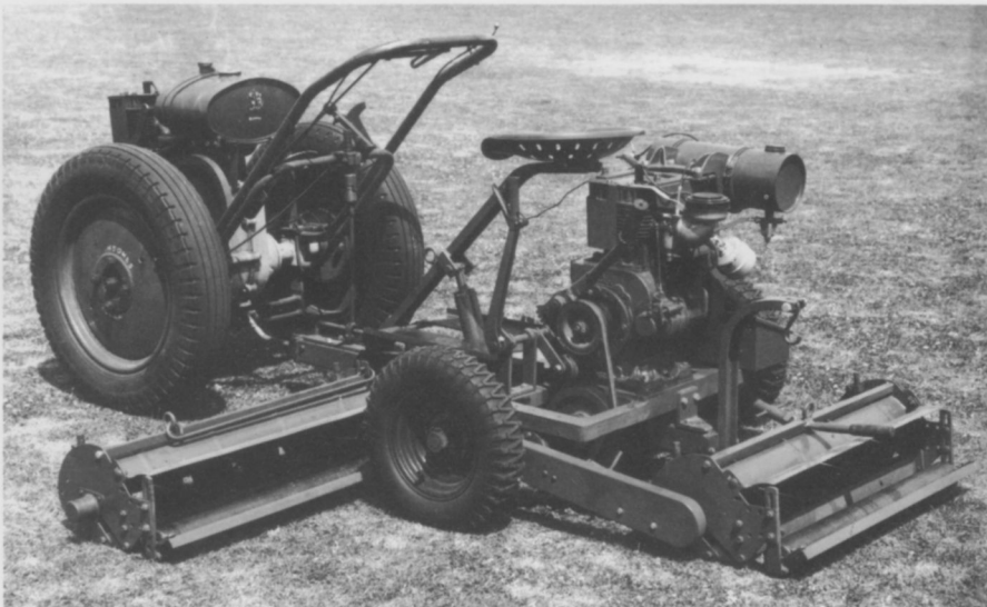
The Auto-Triple solved the problem of driving the cutting units by using a separate motor to that used for propulsion
