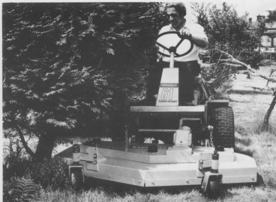
Illustrating the new offset head for the Ransomes 61 Rider Rotary enabling it to cut under shrubs. This new head also has a rear grass discharge as an alternative to a side discharge
