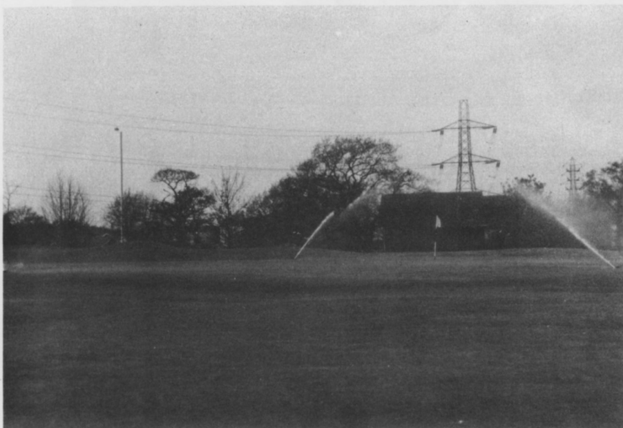
Sectoring Perrot Pop-up sprinklers LVZEW, 7mm nozzle, showing droplet precipitation, providing green coverage well clear of the playing area.
