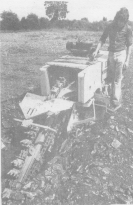
Davis Task Force 500 Trencher which was used during the construction of a golf course in North Staffordshire, on which both the mains drains and greens drains trenches were cut with the machine for the installation at that time of regular clay pipes.
