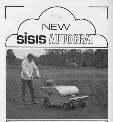
The new SISIS Autocrat is the ideal aerator for all fine turf areas — golf greens, bowling green, etc. The Autocrat gives fast coverage because of its great manoeuvrability (turns in its own length) its 3 ft. width and its speed of operation. A 600 sq. yd. golf green can be tined in 30 minutes and an average bowling green in  $1\frac{1}{2}$  hours.
