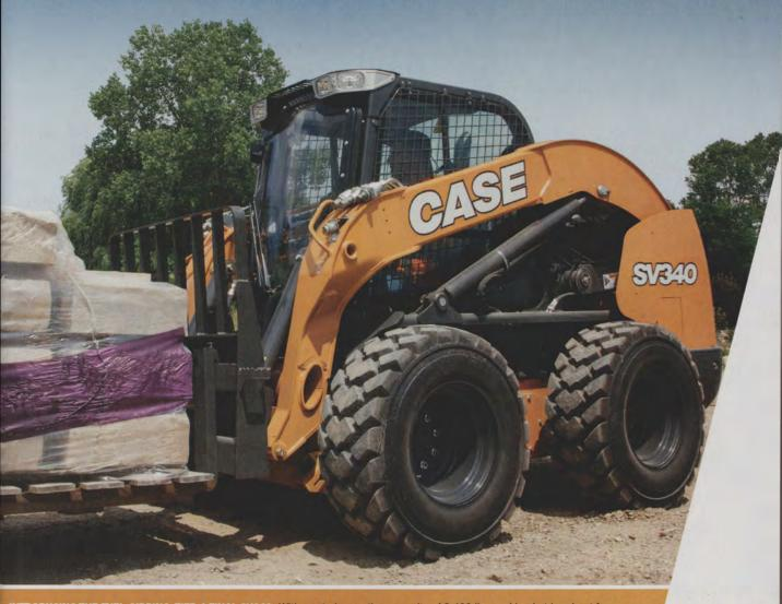
INTRODUCING THE FUEL-SIPPING, TIER 4 FINAL SV340. With a rated operating capacity of 3,400 lbs. and bucket breakout force of 9,531 lbs., the SV340 is a productivity monster. The SV340 runs virtually all attachments with better handling and performance thanks to superior high-flow auxiliary options. Add to that a host of other features and you've got one mean machine that will change the way work gets done on your construction site. Learn more at CaseCE.com/SV340
