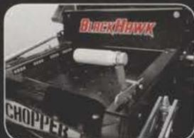
**OCDC** – Foot-operated discharge chute to control grass clippings
