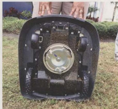
The mower features a cutting width of 8.7 inches with a height range of 0.8 to 2.4 inches.
