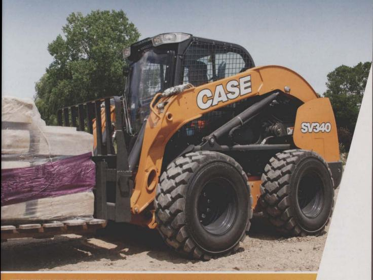
INTRODUCING THE FUEL-SIPPING, TIER 4 FINAL SV340. With a rated operating capacity of 3,400 lbs. and bucket breakout force of 9,531 lbs., the SV340 is a productivity monster. The SV340 runs virtually all attachments with better handling and performance thanks to superior high-flow auxiliary options. Add to that a host of other features and you've got one mean machine that will change the way work gets done on your construction site. Learn more at CaseCE.com/SV340
