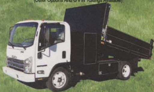
Isuzu NPR HD with 12' Dump Body 297 HP Gas Engine, Automatic Transmission, 14,500 lb. GVWR, 19.5 Tires, AM/FM CD Player, A/C, P/S, Power Windows & Locks, Tilt Wheel, Tow Package & Brake Control, (Other Options And GVW Ratings Available)
