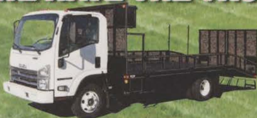
Isuzu NPR with 19' Dovetail Landscaper Body 297 HP Gas or 210 HP Diesel Engine, Automatic Transmission, 12,000 lb. or 14,500 lb. GVWR, Exhaust Brake (Diesel Only), AM/FM CD Player, A/C, P/S, Power Windows & Locks, Tilt Wheel, (Other Options And GVW Ratings Available)
