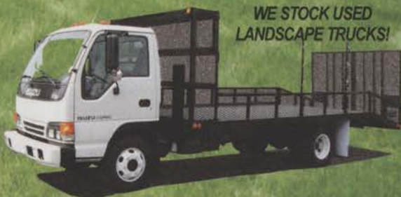
Isuzu NPR HD 4 Door with 19' Dovetail Landscaper Body 297 HP Gas or 210 HP Diesel Engine, Automatic Transmission, 14,500 lb. GVWR, Exhaust Brake, AM/FM CD Player, A/C, P/S, Power Windows & Locks, Tilt Wheel (Other Options And 12,000 lb. GVWR Gas Available)
