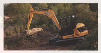
clamp, called the Pro-Clamp. It provides multiple positions for the clamp tip and an alternative tip for that clamp structure to help contractors with a wider variety of tasks.
