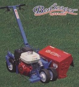
Model BE400 defines borders with a mulch retaining wall 2", 3" or 4".
