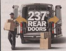
The Transit van is available with the best-in-class maximum rear cargo door opening height. The doors open a full 237° and the floor is as low as 28 inches.\*\* It's all about making loading and unloading easier. No matter what your business is.
