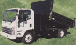
297 HP Gas Engine, Automatic Transmission, 14,500 lb, GWR, 19.5 Tires, AMFM CD Player, A/C, P/S, Power Windows & Locks, Tilt Wheel, Tow Package & Brake Control. Other Options And GVW Ratings Available)
