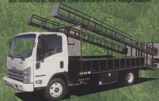
Isuzu NPR with 19' Custom Irrigation Body 297 HP Gas or 210 HP Diesel Engine, Automatic Transmission, 12,000 lb. or 14,500 lb. GVWR, Exhaust Brake (Diesel Only), AM/FM CD Player, A/C, P/S, Power Windows & Locks, Tilt Wheel, (Other Options And GVW Ratings Available)
