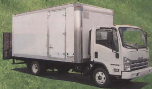
Isuzu NPR with 18' Enclosed Landscape Body 297 HP Gas Engine, Automatic Transmission, 12,000 lb. GVWR, AM/FM CD Player, A/C, P/S, Power Windows & Locks, Tilt Wheel, Split Dovetail Ramp, Side Door, (Other Options And GVW Ratings Available)
