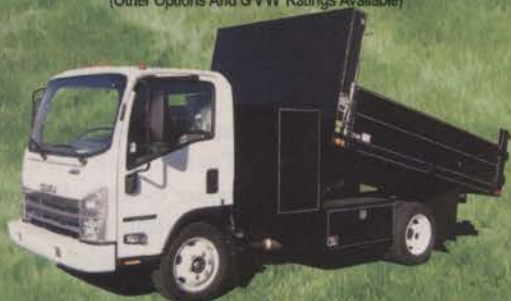
Isuzu NPR HD with 12' Dump Body 297 HP Gas Engine, Automatic Transmission, 14,500 lb. GVWR, 19.5 Tires, AM/FM CD Player, A/C, P/S, Power Windows & Locks, Tilt Wheel, Tow Package & Brake Control, (Other Options And GVW Ratings Available)
