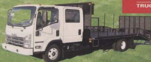
Isuzu NPR HD 4 Door with 19' Dovetail Landscaper Body 297 HP Gas or 210 HP Diesel Engine, Automatic Transmission, 14,500 lb. GVWR, Exhaust Brake, AM/FM CD Player, A/C, P/S, Power Windows & Locks, Tilt Wheel (Other Options And 12,000 lb. GVWR Gas Available)
