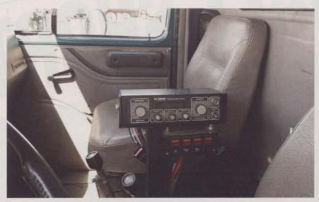
Computerized in-cab controls allow you to put down the proper application rates for the de-icing materials so you can regulate the amount of material that gets applied to the surface.
