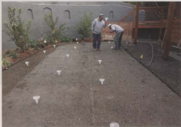
Gardenworks crew members perform a catch can test.
