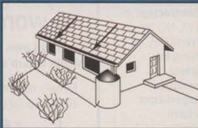
Water rolls down the roof, into the downspouts and falls in a central tank.
