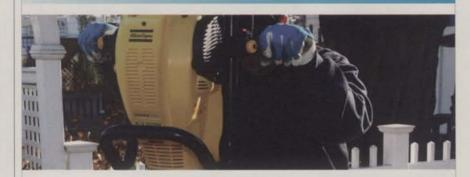
Atlas Copco Cobra Pro — an efficient, gas-powered tool that digs fencepost holes, cuts asphalt, drives tent stakes, and even tamps ground.
